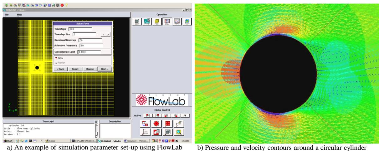
**Figure 3: Computational modelling input screen and results**
