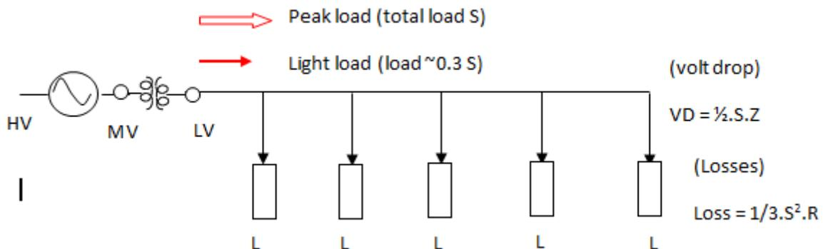
Figure 3: Approx. Uniformly Loaded Feeder – No Storage or Generation (Base Case)
