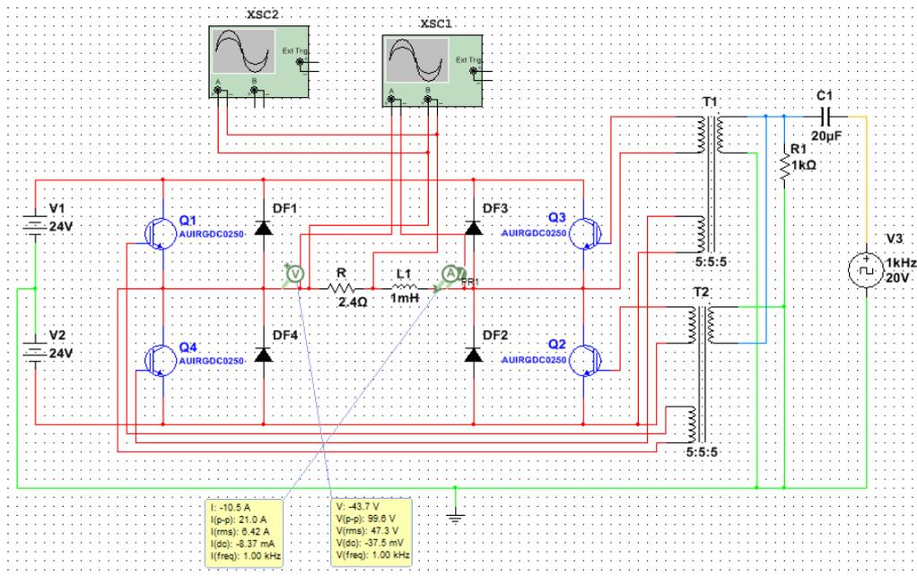
Figure 4: Multisim model of a Single-Phase Full Wave Inverter with Resistive and Inductive Load (Output blocks showing voltage and current outputs) (Kamal 2018).
