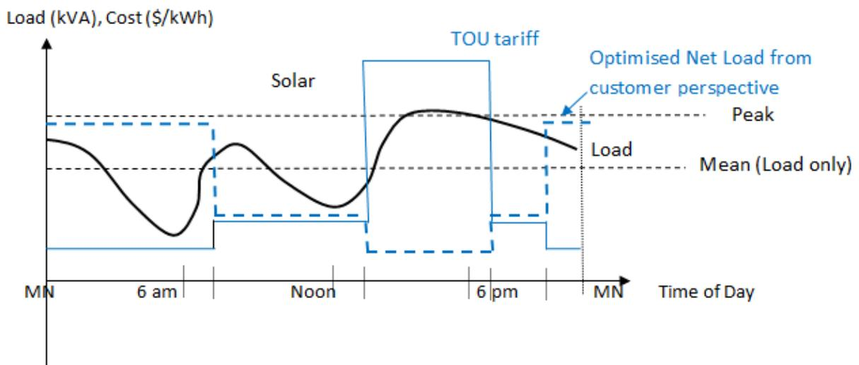
**Figure 8:** Daily Net Load +/- Storage Curve Optimised from Customers' Point of View
