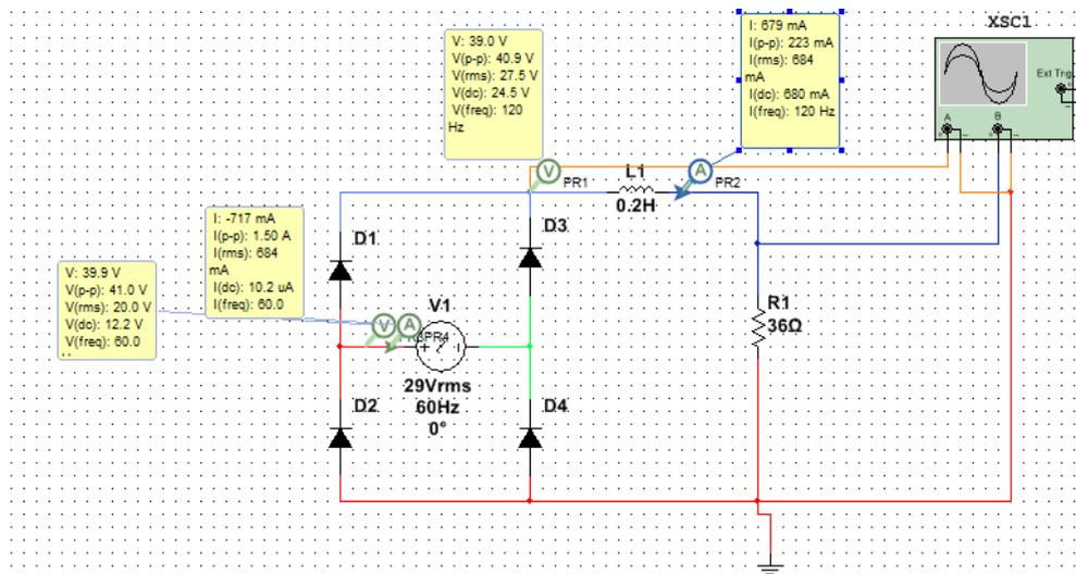
**Figure 2:** Multisim model of a Single-Phase Full Wave rectifier with Resistive and Inductive Load (Rao & Prakash 2018).
