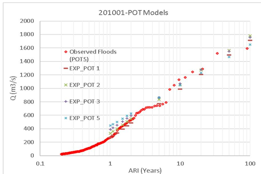
**Figure 1: Flood estimates for Station 201001 in NSW using POT models based on 54 years' recorded data (1958-2011)**
