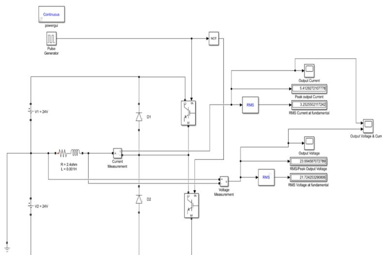
**Figure 3:** Simulink model of a Single-Phase Full Wave Inverter with Resistive and Inductive Load (Output blocks showing voltage and current outputs) (Kamal 2018).
