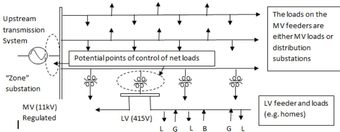
Figure 2: Typical Medium and Low Voltage Ring Main Feeder System layout.
