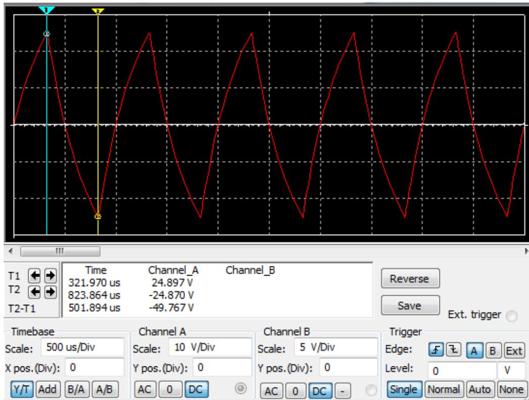
**Figure 8:** Full Bridge (LR load) Output Current waveform – Multisim (Kamal 2018).
