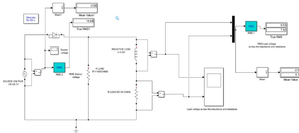
**Figure 1:** Simulink model of a Single-Phase Half Wave rectifier with Resistive and Inductive Load (Rao & Prakash 2018)
