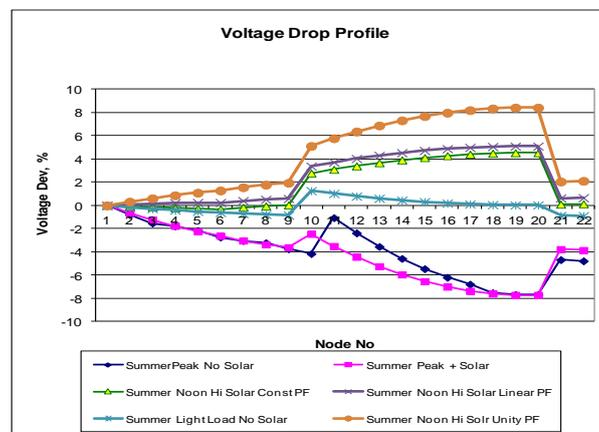
**Figure 5:** Generic 10-node Radial Feeder Voltage Profile
