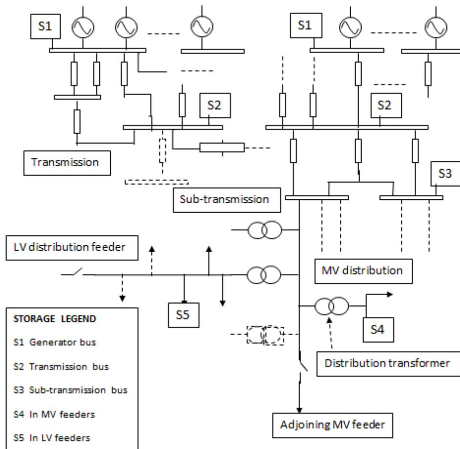
**Figure 1:** Typical Power System Arrangement and Possible Storage Locations (transformers in the transmission and sub-transmission omitted for clarity)
