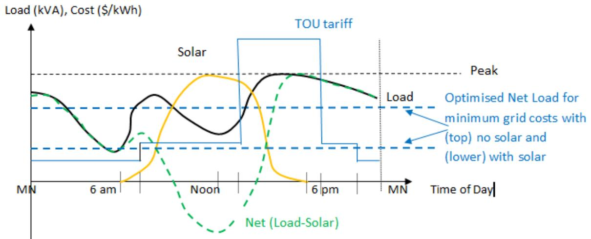
**Figure 7:** Daily Load Curve with Significant Storage. A flat net load curve will incur uneven tariff charges
