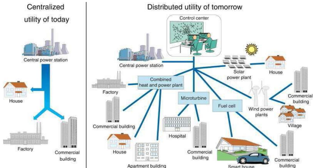
**Figure 1:** (a) Traditional Power Systems (b) Distributed Power Systems of future
