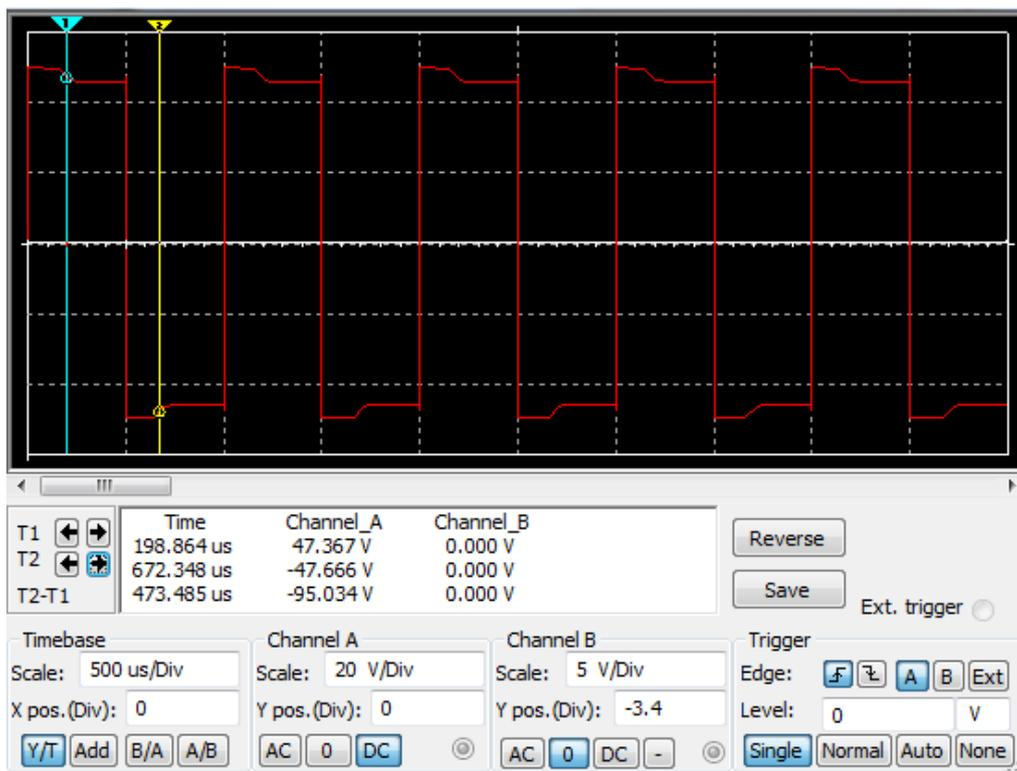
Figure 7: Full Bridge (LR load) Output Voltage waveform – Multisim (Kamal 2018).
