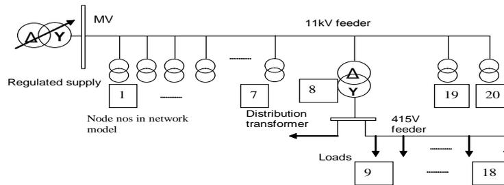
**Figure 4:** Generic "10-node + 10-node" Radial Feeder Model
