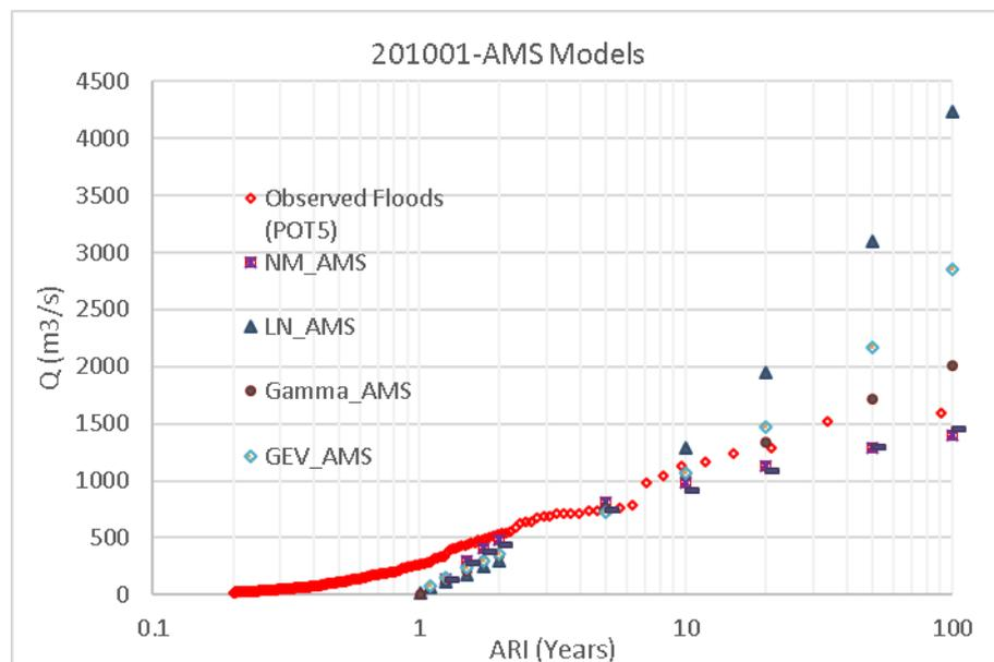
**Figure 2: Flood estimates for Station 201001 in NSW using AMS models based on 54 years' recorded data (1958-2011)**
