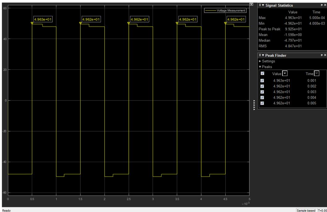
Figure 5: Full Bridge (LR load) Output Voltage waveform – Simulink (Kamal 2018).
