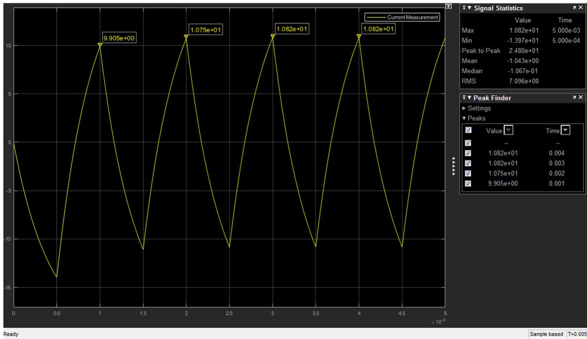
Figure 6: Full Bridge (LR load) Output Current waveform – Simulink (Kamal 2018).
