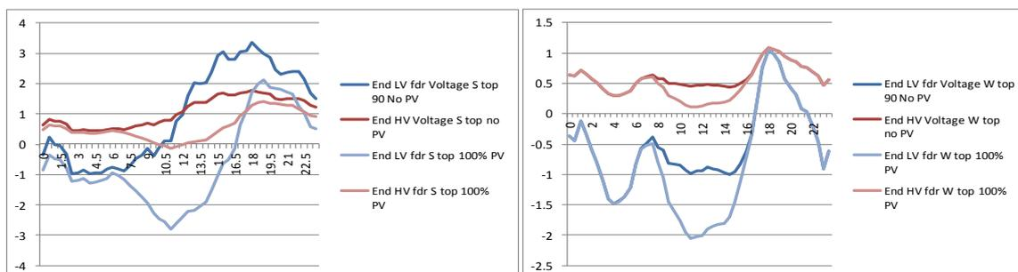
**Figure 6:** Hourly Feeder Extremity Voltage Drop for CSIRO "Future Grid" "50 Homes" Data
