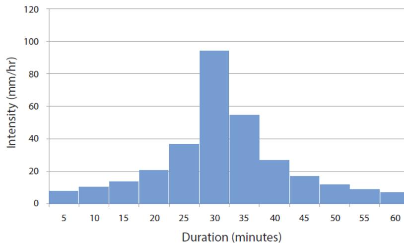
**Figure 6.** Hyetograph plot for 5 minute duration and 10 year ARI, Qatar, using alternating blocking method
